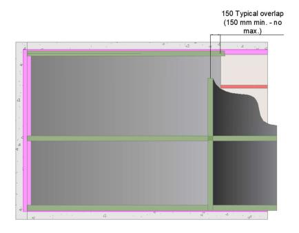
Once the joints have been formed and the membrane is temporarily secured, apply the correct illbruck tape to seal the overlap. The tape should be wrinkle and bubble free, and consolidate the bond with a seam roller.
