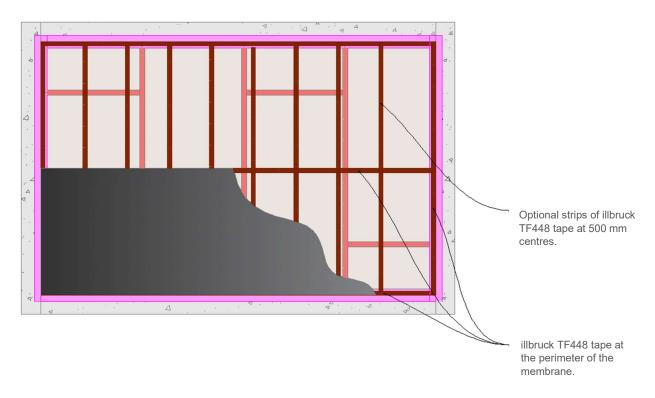
For low to medium wind loads the double sided tape should be applied around the entire perimeter of the membrane. For higher wind loads, the bond can be further enhanced by installing vertical strips of TF448 High Performance Bonding Tape at 500 mm centres.
